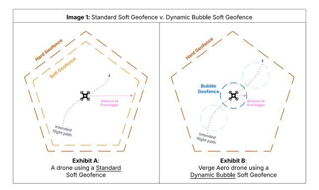
Verge Aero's dynamic bubble soft geofence keeps a drone within a few meters of its target position, rather than allowing it to potentially veer far off course before a mission is terminated. If an individual drone deviates from its flightpath enough to breach its "bubble" radius, it lands immediately by descending vertically in a controlled manner until it reaches the ground and the motors turn off.
